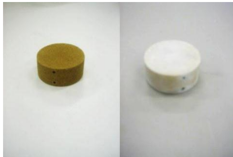
Figure 5: Sand Specimen and Reference Material used for Experimentation
